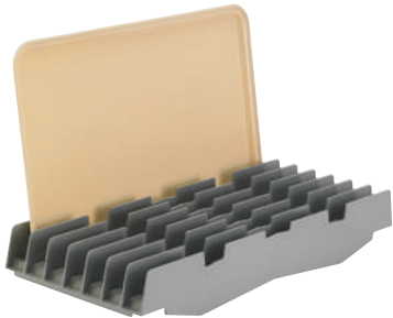
Modular 7-slot rack can be ordered separately to customize a drying and storage rack. Made of highly durable ABS plastic. Slots are spaced 1 5/16" wide and dividers are 2 1/2" high.
